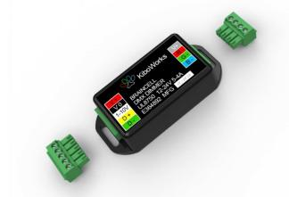
Affectionately called the BrainCell. This unit will accept DMX512, 0-10V, or Fiber DMX data and output 3 independent channels of pulse width modulated signals with a common class 2 V+. Advanced features include special ordered built in effects selected by a button.
